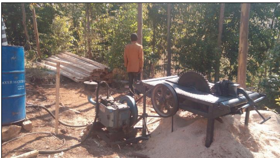
Figure 13.4 Layout of a dingdong saw: table, blade, engine, and drive belt
