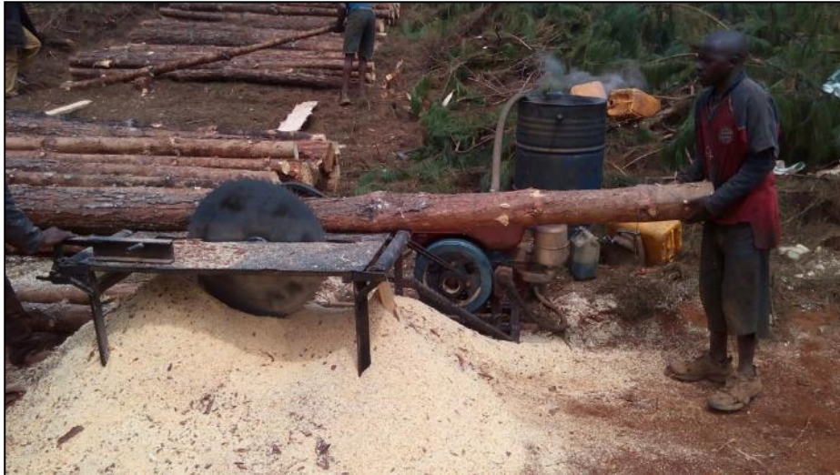
Figure 13.3 Operating a dingdong saw
