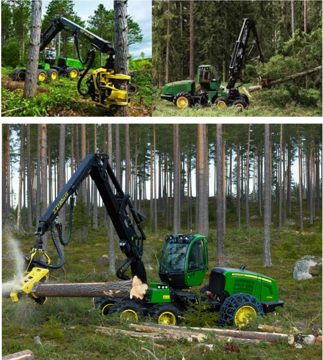
Figure 10.1 The harvester takes hold of a standing tree, cuts its trunk, strips the branches as it drops it on the ground
