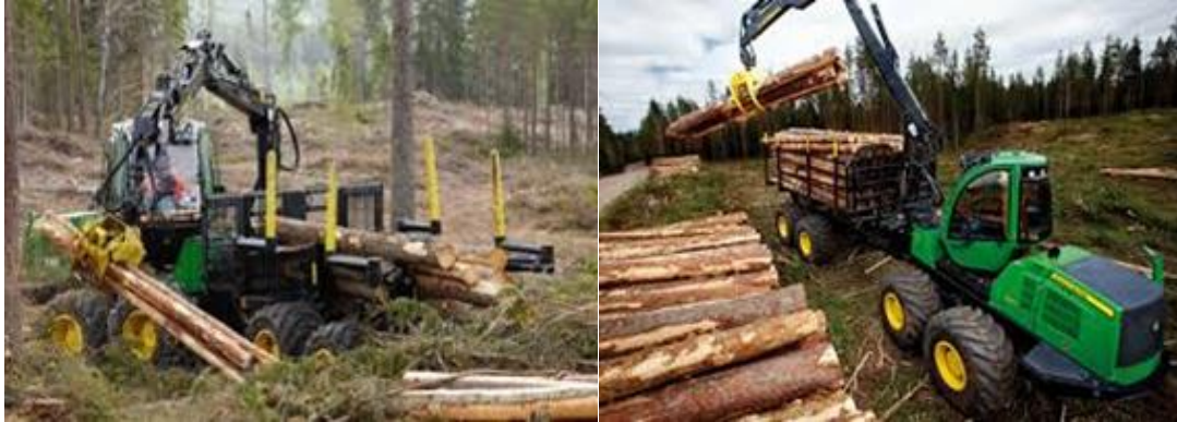
Figure 10.3 A forwarder then the logs from the forest floor and stacks them at the side of a road for collection
