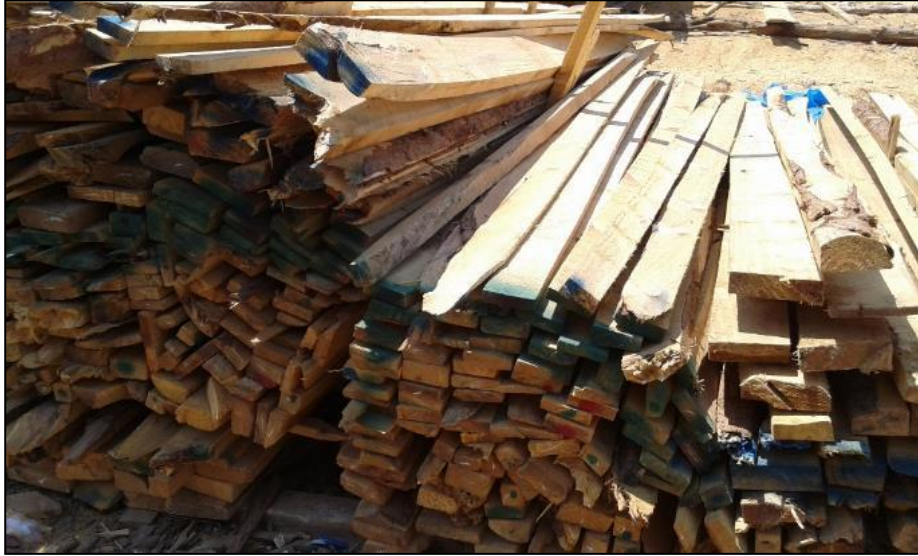
Figure 13.5 Poor-quality eucalyptus lumber with twists and cracks
