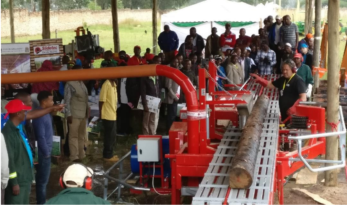
Figure 33 Precision-sawn wood, produced here by the multi-rip saw of the FWITC, improves yields and product quality
