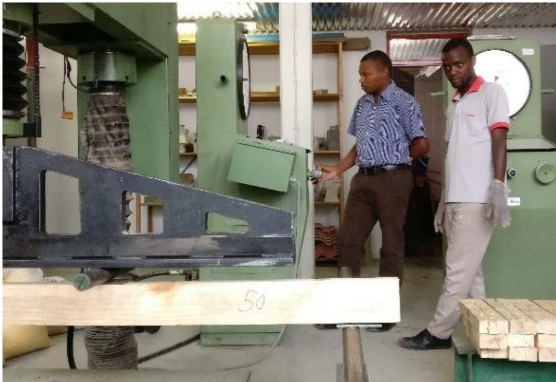
Figure 13 Destructive testing done at the TBS to establish the strength values of sawn wood
