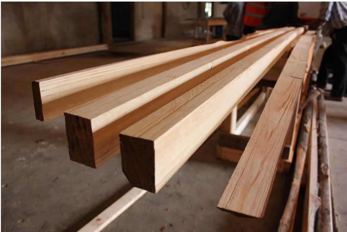
Figure 33 Precision-sawn wood, produced here by the multi-rip saw of the FWITC, improves yields and product quality
