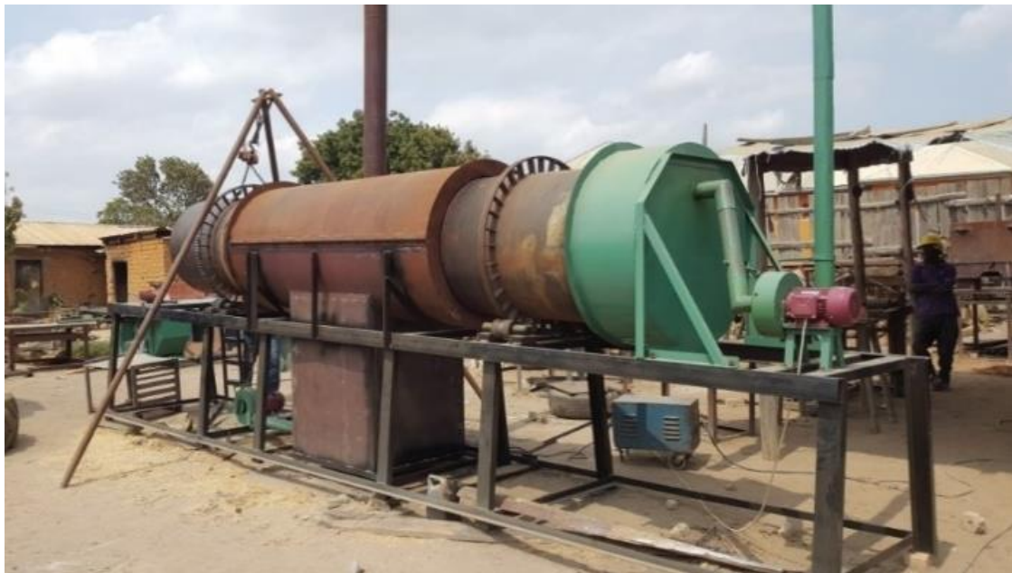
Figure 35 Sawdust carbonizer being assembled for the FWITC at a workshop in Mafinga
