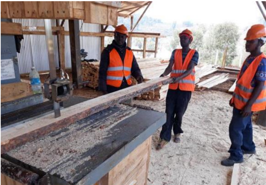
Figure 31 Upgraded vertical band saw technology with improved sawing precision, productivity, safety and working conditions
